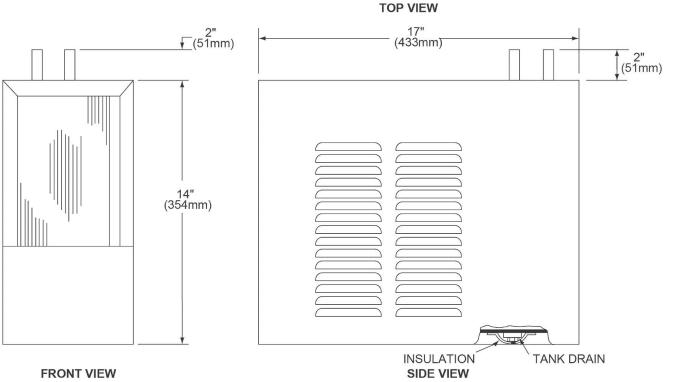
NOTE: It is important to insure proper ventilation. If this remote chiller is physically placed against barrier or in enclosure of any kind, 4" (102mm) air space must be allowed on all sides.
